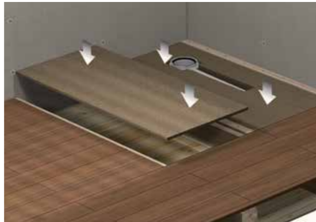
4. Fix timber panels to support ensuring a level deck at joist height.
