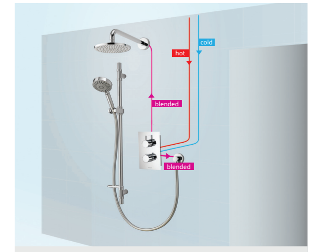
Divert outlet with adjustable and wall mounted drencher heads
