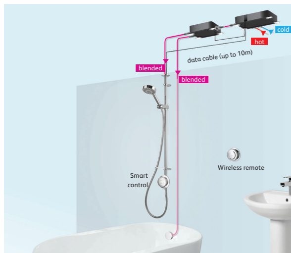
Exposed shower with bath overflow filler
