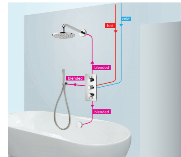
3 way outlet with hand shower, wall mounted drencher head and bath fill
